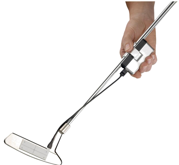
Align ZENIO in heel-toe direction
